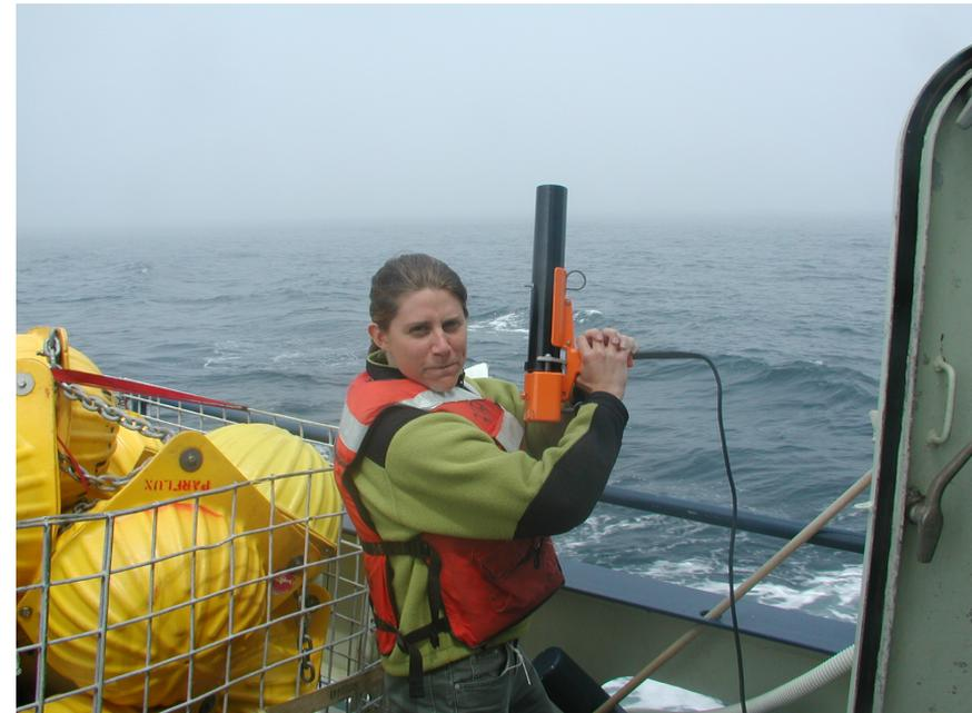
XBT: Expendable bathythermograph. Measure temperature and depth to ~1000 m
