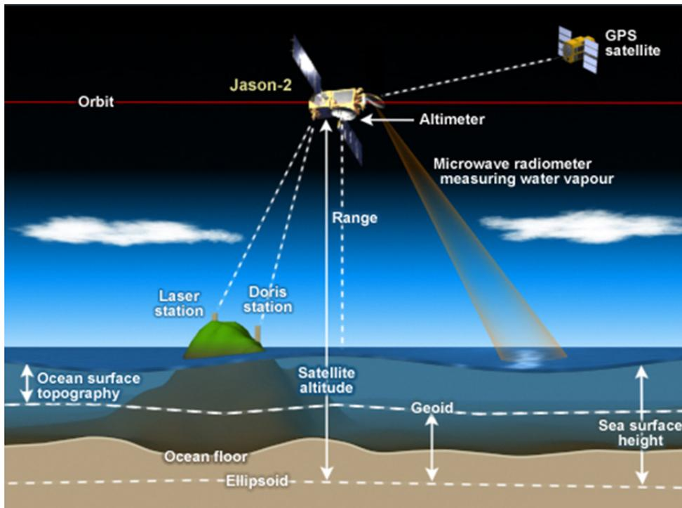
The altimeter measures the distance to the surface,  $R_{alt}$ , and its own altitude,  $H_{alt}$  (ref. ellipsoid). From them we get the sea surface height (SSH):
