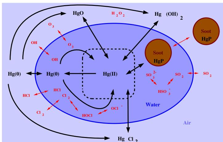
Figure 17: Chemical mechanism for mercury developed by Yelva Roustan in his PhD work on the basis of state-of-the-science models.
