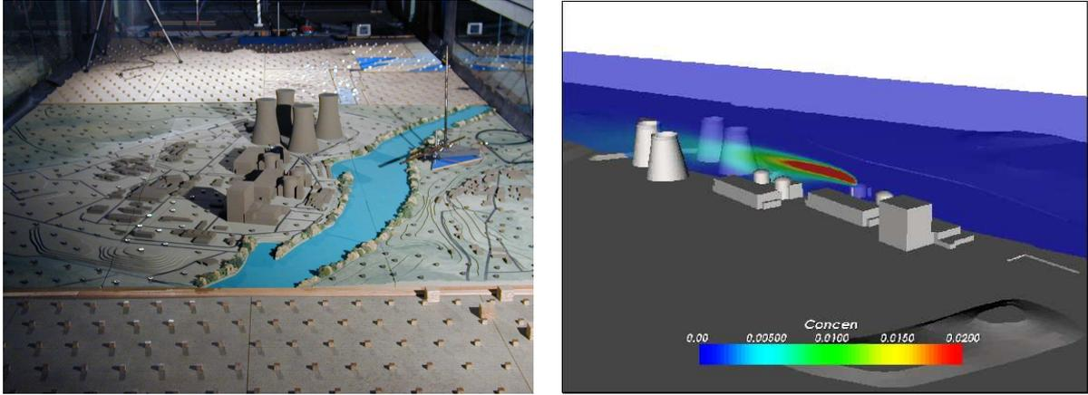
Figure 3: Top left: view of the wind tunnel experiment (ECL/IRSN). Top right: simulated concentration field. Bottom: comparison of concentration profiles between wind-tunnel data, Mercure\_Saturne and ADMS 3.0 simulations for the release on the chimney (vertical profile at 400 m in built-up area) (Emmanuel Demael PhD Thesis).
