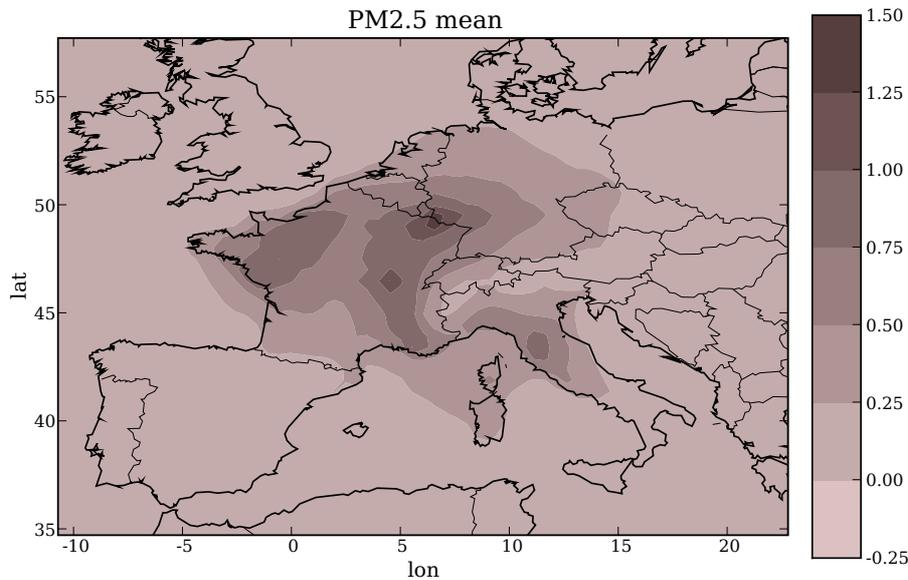
Figure 19: Impact for the year 2005 of the emissions from the French thermal power plants (EDF and SNET). The target is  $PM_{2.5}$ . The indicator is a relative impact computed in % by comparing a reference simulation and a simulation without the emissions.
