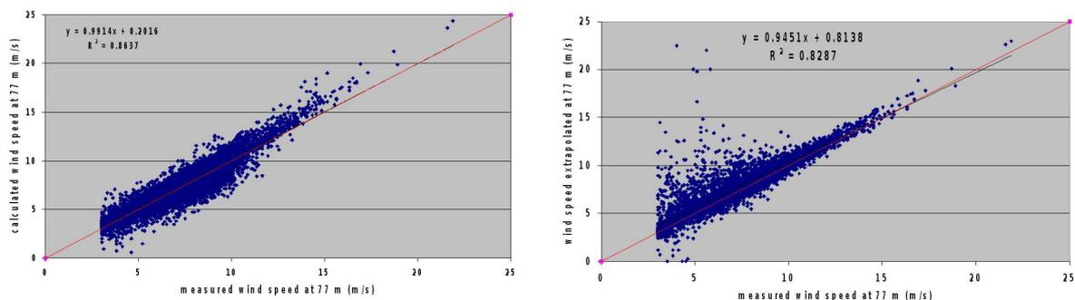
Figure 33: Comparison between computation and measurement of wind speed at 80 m, for a one-year data set (December 2004 to December 2005), with two methods: one using normalized vertical profiles measured by sodar (left panel), one using a simple power law (right panel).
