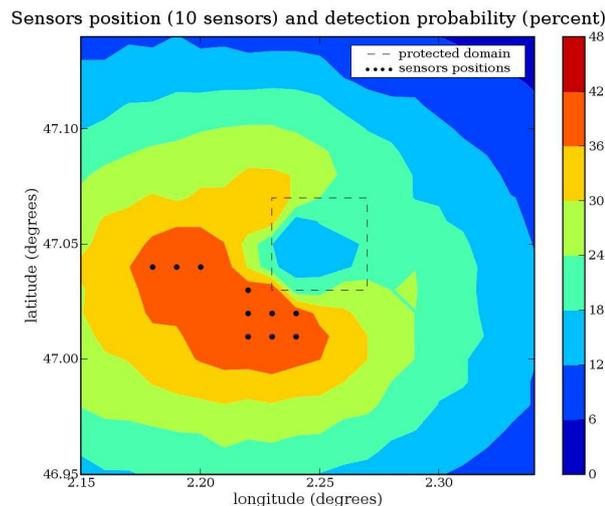
Figure 31: Network design on a battlefield (regional scale). Map of detection probability at regional scale for all possible sensors, as well as the sensors positions for the ten sensors having the best detection probability.
