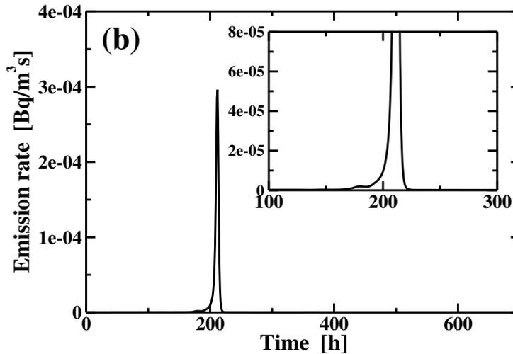
Figure 24: Reconstructed profiles of an accidental release of Cs-137 in Algeciras, Spain, using especially devised cost-function. Some  $[2.96 \times 10^{11}; 2.96 \times 10^{12}]$  Bq released between 01:00 and 03:00 UTC on 30 May 1998. Time of the release corresponds to 215-217 on the horizontal axis. Reconstructed activity:  $2.96 \times 10^{12}$  Bq.
