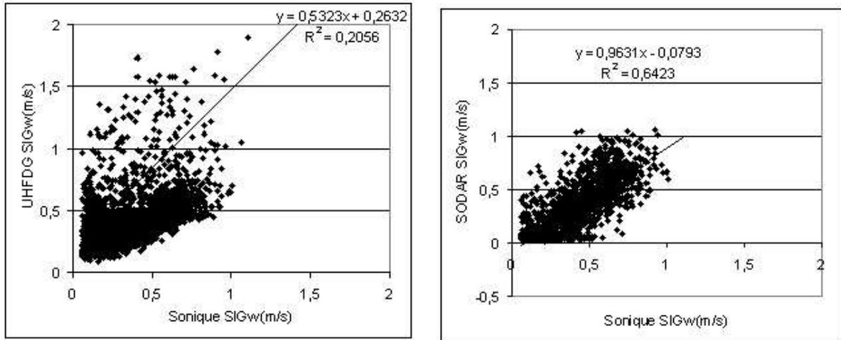
Figure 34: Comparison between spectral width measured on UHF vertical beam and standard deviation of vertical velocity measured by sonic anemometer (left panel). Also between standard deviation of vertical velocity measured by sodar and sonic anemometer (right panel).
