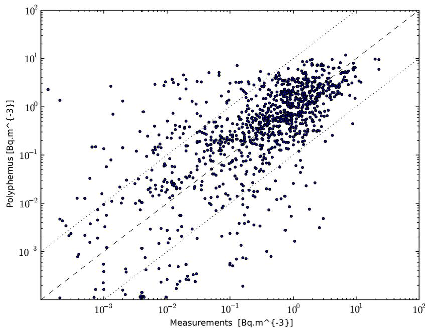
Figure 20: Model-to-data comparison (scatter plot) for cesium 137 for the first two weeks after the Chernobyl release.
