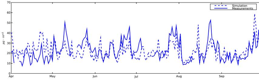
Figure 10: Time series of measured versus simulated  $PM_{10}$  concentrations at station Gennevilliers (Paris suburb) for April-October 2001.
