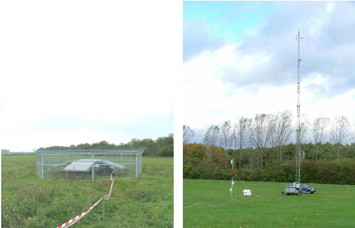
Figure 35: Views of the radar UHF (left) and the 30-meter mast (right) installed on the SIRTA site.
