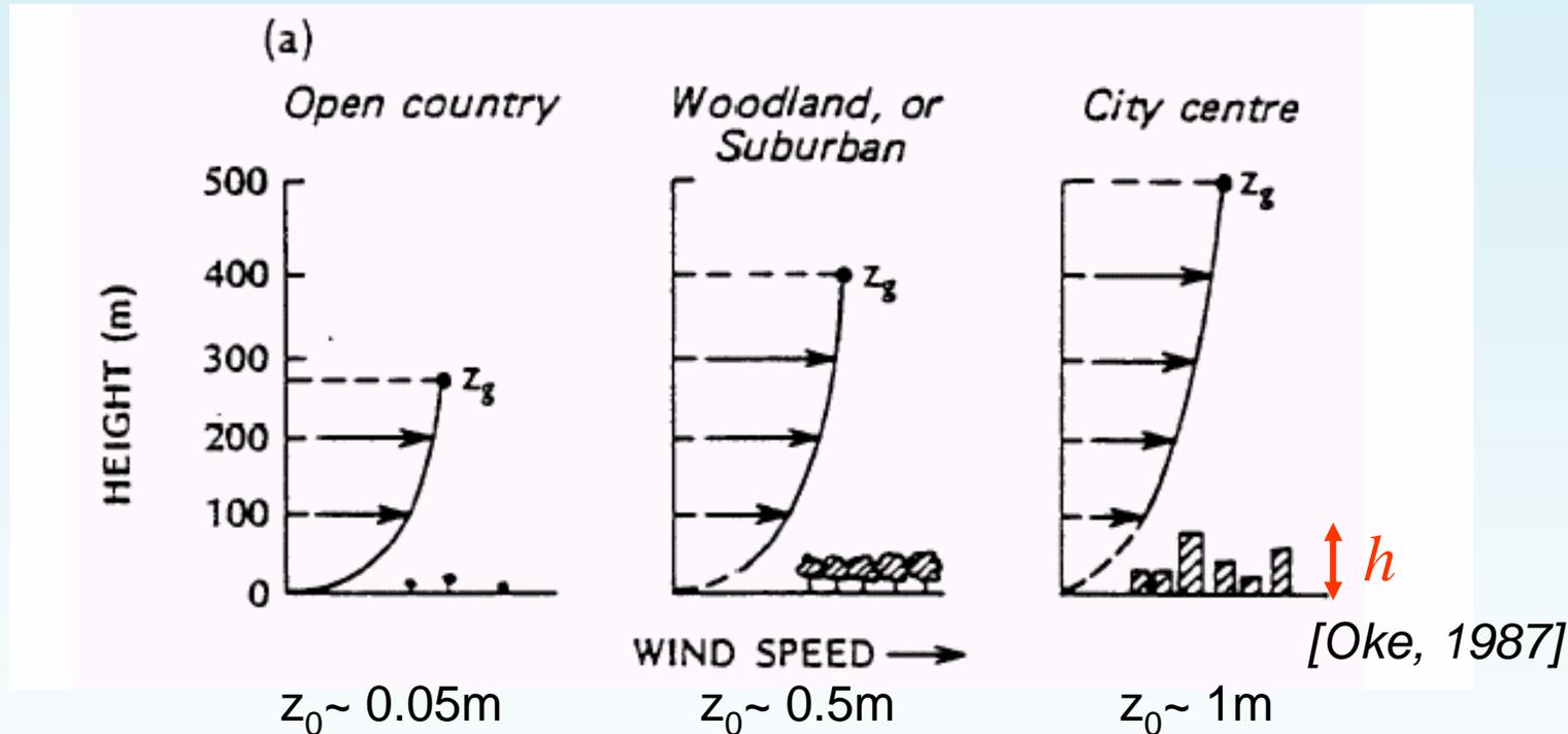
$$\left| \begin{array}{l} \bar{u}(z) = \frac{u_*}{\kappa} \ln\left(\frac{z-d}{z_0}\right) \quad z > 2h \\ \bar{u}(z) = 0 \quad z = z_0 + d \end{array} \right.$$
